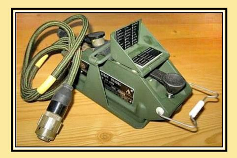
This pamphlet is a follow-up of WftW Pamphlet series No. 5, 'Key and Plug Assemblies Pt. 1', which was primarily associated with the British 'Key W.T. 8 Amp.' Shown in part 2 are hand speed Morse keys used with the British Army HF radios in the Larkspur and Clansman range, with the emphasis of being an assembly with a lead and plug, and leg straps. These Morse keys were often incorporated in a remote control assembly used for local and remote keying.
